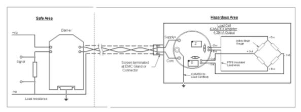
The barrier shown above limits the amount of electrical energy that can be transferred into the hazardous area, thereby preventing the ignition of a flammable atmosphere in the event of a fault condition occurring.
