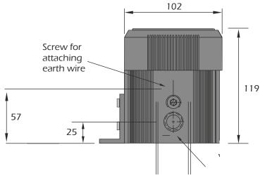
Two M20 x 1.5 cable entries (model number suffix M) or two 1/2 inch NPT cable entries (model number suffix N)
