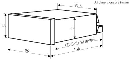
Panel cutout should be 92mm wide x 45mm high, +1mm, -0mm 1/8 DIN. Depth behind panel 125mm max, including cables.
