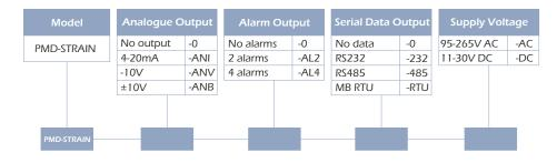
Example - PMD-STRAIN display with 4-20mA output, 2 alarms, RS485 output and 110V AC powered Order code will be: PMD-STRAIN-ANI-AL2-485-AC
